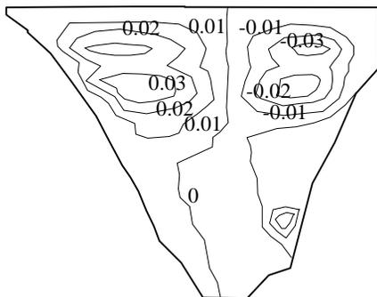
**Fig. 13** Contours of displacements in the X direction of the slab for reservoir filling (m)
