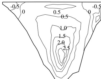
**Fig. 16** Contours of stresses on slab in the direction along the dam axial for reservoir filling (MPa)
