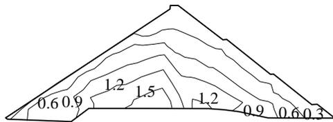
**Fig. 11** Contours of major principal stresses of the dam during reservoir filling (MPa)
