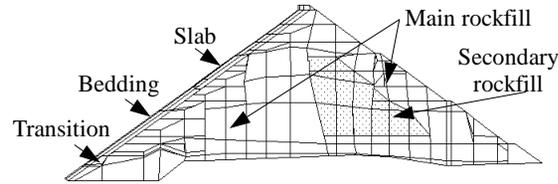
**Fig. 2** Maximum cross section of the dam
