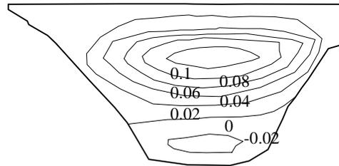
**Fig. 7** Contours of displacements in the X direction
