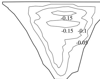
**Fig. 14** Contours of displacements in the Z of the slab reservoir filling (m)
