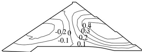
**Fig. 3** Contours of horizontal displacements of the dam during construction (m)
