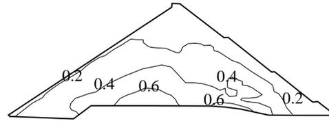
**Fig. 12** Contours of minor principal stresses of the dam during reservoir filling (MPa)
