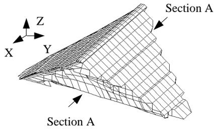
**Fig. 1** Three-dimensional finite element discretization of Yutiao dam
