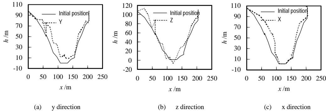
Fig. 17 Displacements of peripheral joints during reservoir filling
