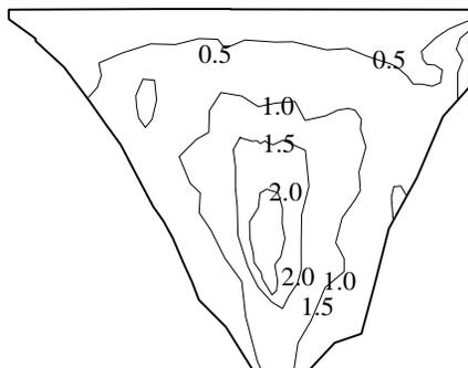
**Fig. 15** Contours of stresses on slab in the direction along the dam slope for reservoir filling (MPa)
