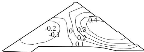
**Fig. 9** Contours of displacements in the y direction
