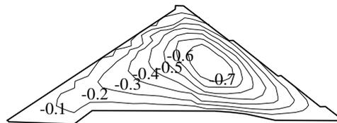
**Fig. 4** Contours of vertical displacements of the dam during construction (m)
