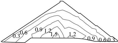
**Fig. 5** Contours of major principal stresses of the dam during construction (MPa)
