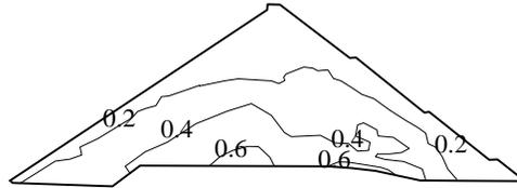
**Fig. 6** Contours of minor principal stresses of the dam during construction (MPa)
